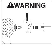
Always disconnect air from the nailer whenever servicing! During maintenance, a nailer connected to air may fire accidentally, causing serious personal injury!
